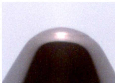
Figure 2 — Correct shape of the scratching tip
