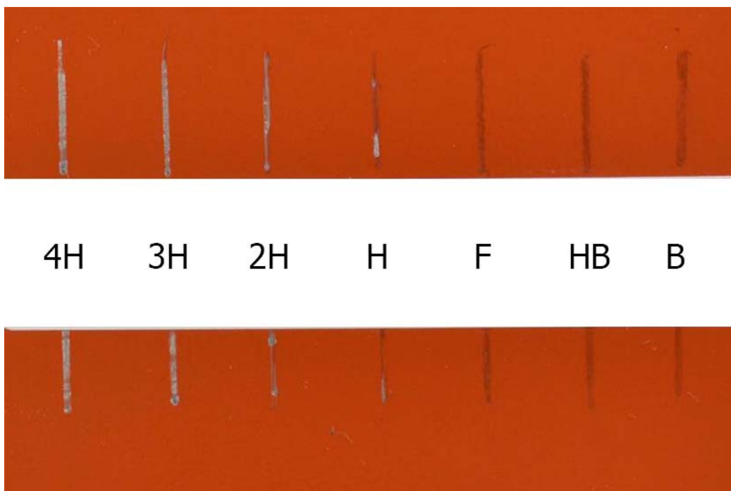
FIG. 2 Typical Example of Pencil Test
