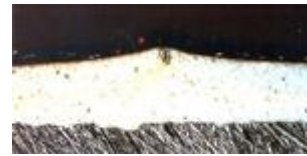
Metal Particle in E-Coat
