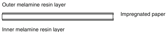
Figure 15 General structure of melamine papers.
