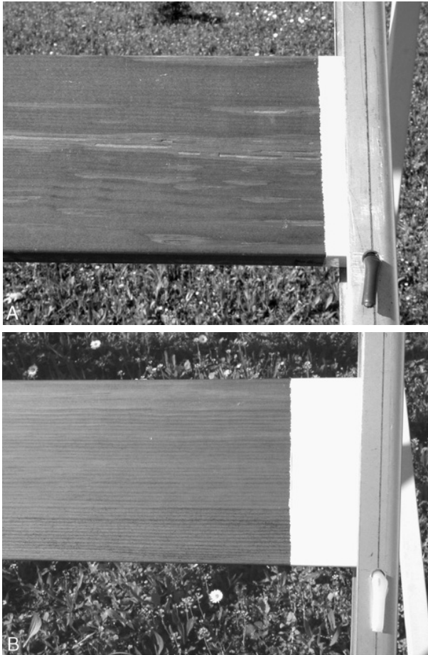
Figure 7 Two different coatings after 1-year exposure according to EN 927-3 (picture from CATAS spa).
